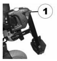
Loosen the fixing mechanism by tapping lightly against the handscrew.
