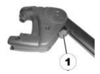
The rubber stop can be screwed in or out (A) or pushed up or down (B).
