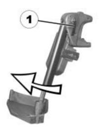
• Use the open-ended spanner to loosen the counternut (1).
