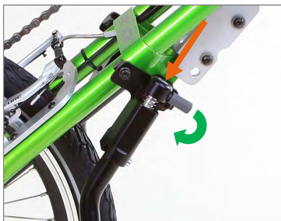
Figure 3: Press down and turn the operating lever
