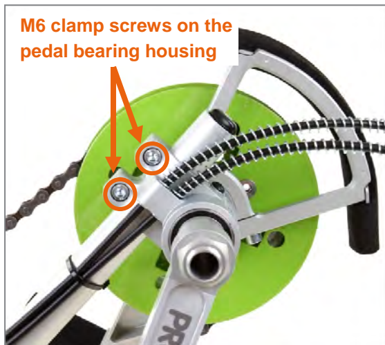
Figure 12: M6 clamp screws on the pedal bearing housing for the height adjustment of the pedal bearing position and the replacement of the pedal bearing support
