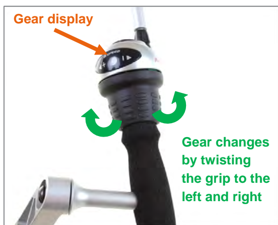
Figure 16: Shifting using the grip shift for the Shimano Nexus Inter8 hub drive
