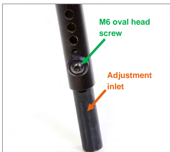
Figure 9: M6 oval head screw and adjustment inlet to adjust the height of the parking stand
