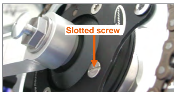
Figure 33: Slotted screw to lubricate
