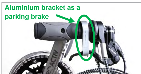
Figure 36: Aluminium bracket as a parking brake
