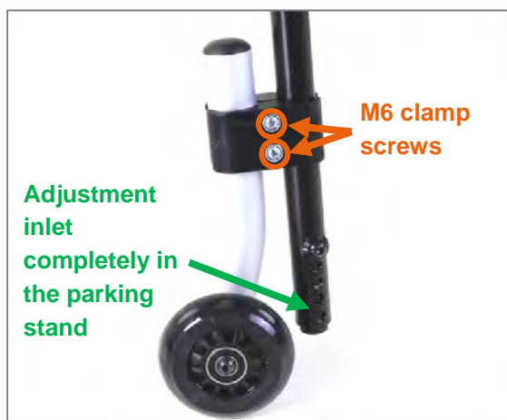
Figure 10: M6 clamp screws in the manoeuvring rollers
