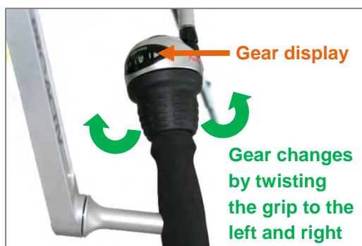
Figure 24: Shifting using the grip shift for the Shimano Nexus Inter8 hub drive
