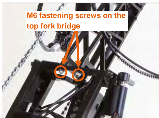
Figure 13: M6 fastening screws on the top fork bridge
