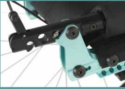
As a standard feature it includes a soft locking mechanism on the backrest so that it doesn't open when folded.
