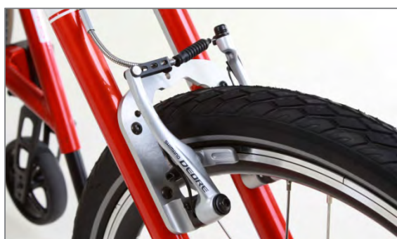
Figure 10: Rim brake connected and cable length set correctly
