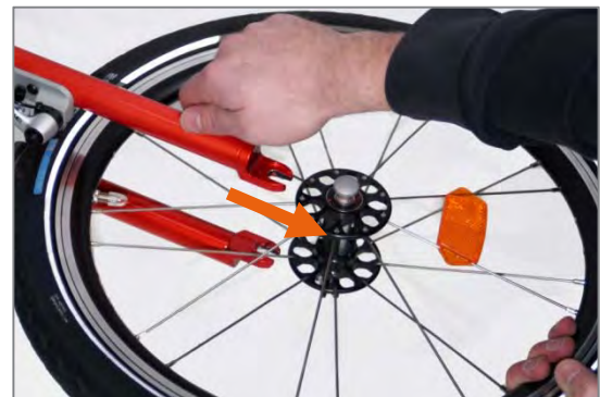
Figure 7: Remove the wheel by pulling downwards
