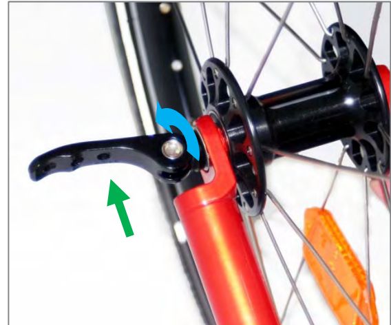
Figure 6: Open and turn quick release
